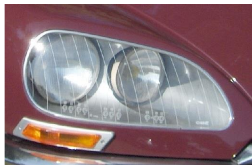
Figure 3: Headlamp on a Citroën DS with European “Sealed beam” configuration
