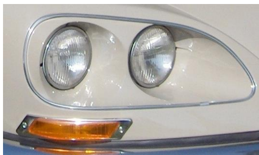
Figure 2: Headlamp on a Citroën DS with U.S. “Sealed beam” configuration
